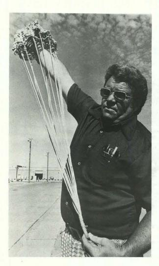
DENNIS CRONIN (1332) displays new 19-in. diameter Kevlar parachute designed for ballistic nosecone recovery.
